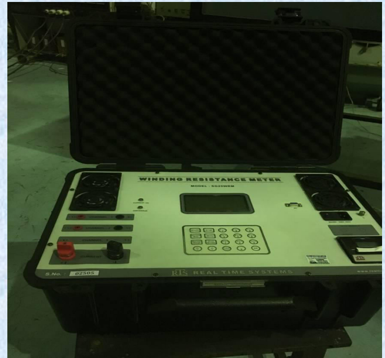
4 – Wire, 2 - Channel Winding Resistance Meter, 0.2 m \Omega - 2000 \Omega , Accuracy 0.2 % FSD
