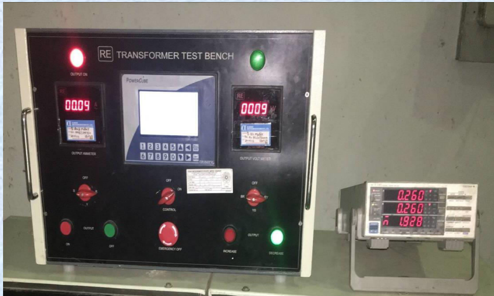
3-Phase Transformer Test Bench, 75 kVA, 2000 V & 52 Amps
